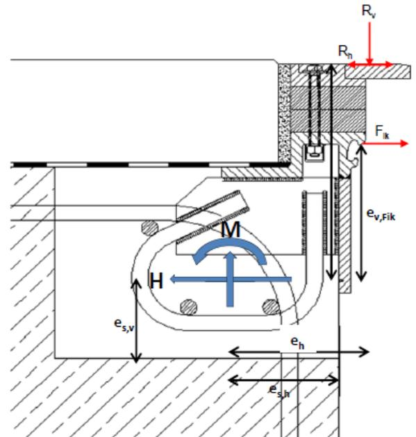
Note: The two lines indicating the forces transferred to the anchorage are taking into account the horizontal loads acting in both directions.
