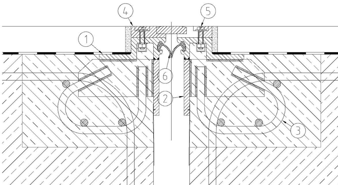
Figure 1: Exemplary cross section of the nosing expansion joint
