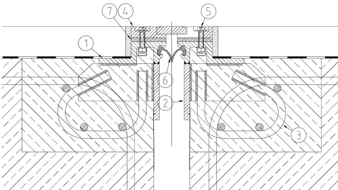
Figure 2: Exemplary cross section of the nosing expansion joint
