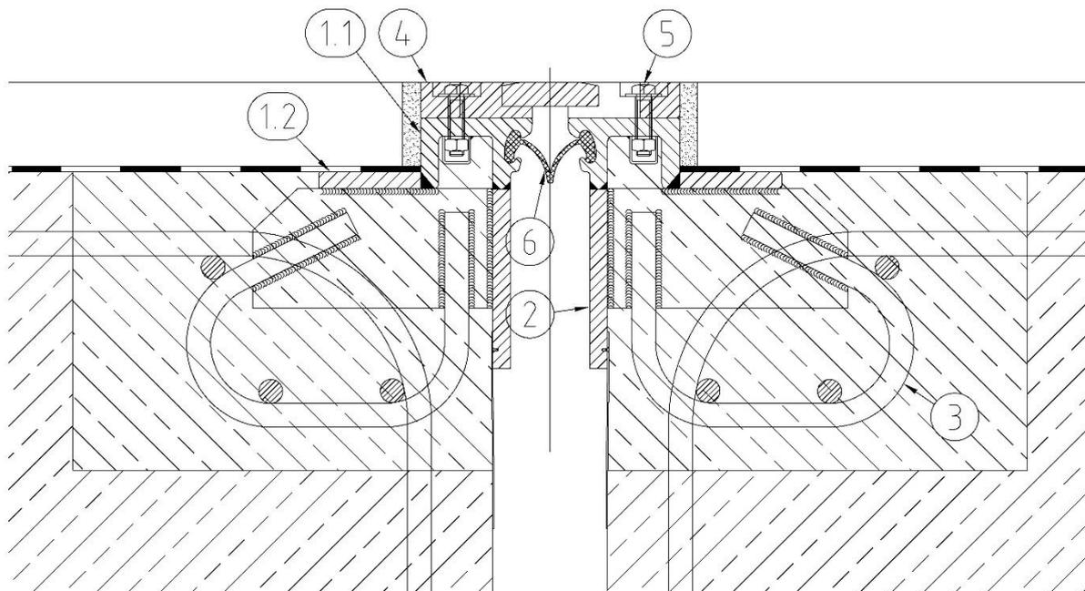
Figure 3: Exemplary cross section of the nosing expansion joint
